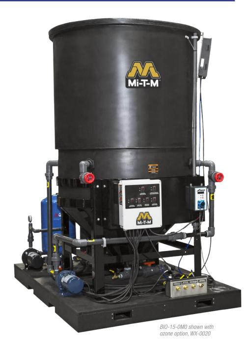
A clarifier acts as a form of pretreatment in many systems and the cone bottom design allows for a greater settling of accumulated solids. These concentrated impurities, often referred to as sludge, will settle in the bottom of the tank for easy removal. Pretreatment makes it easier for wastewater treatment systems to process water with many of the solids already removed.
