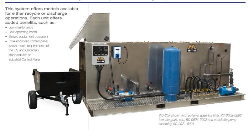
The popular BIO Series System utilizes fixed-film bacteria in conjunction with coalescing media to treat waste water. A variety of tank sizes and flow rates are used to create retention time to treat the wastewater. Oxygen is added to the bacteria in the waste stream by venturi injection system.
