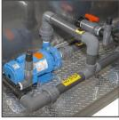
Mazzei® venturi air injection system, 55-0126, sustains beneficial aerobic microbes while preventing bacteria from
