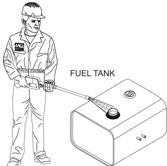
Figure 45. Fuel Tank Cleaning
