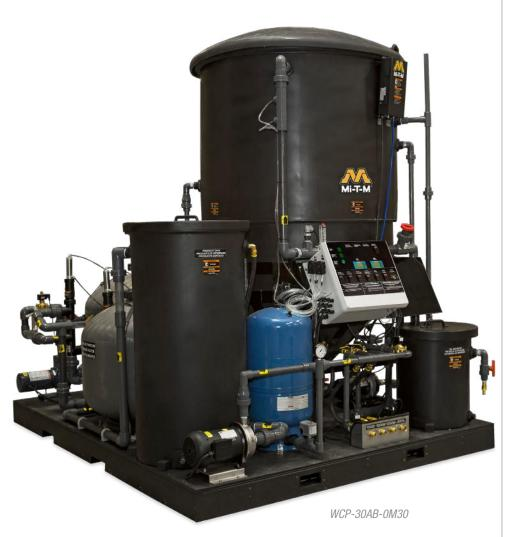
Designed to remove free hydrocarbons and filter water, these systems come standard with pH and ORP injection and are corrosion-resistant when utilizing polymer tanks and recycled plastic skids.
